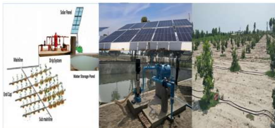
Figure 5. Conceptual layout of solar operated high efficiency irrigation systems
